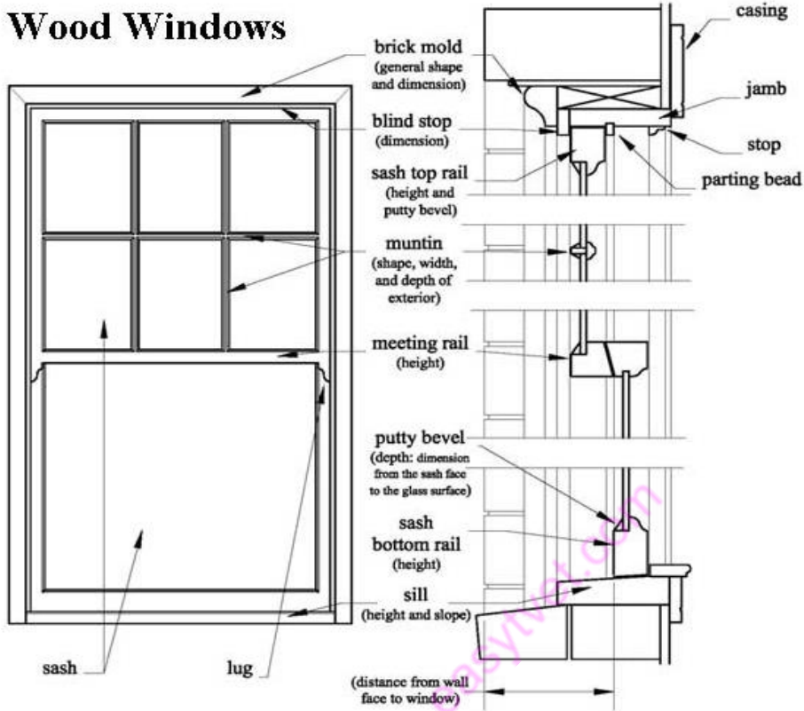
Figure 38 Wood window details
