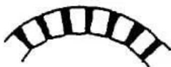
uncut bricks with wedge shaped mortar joints
