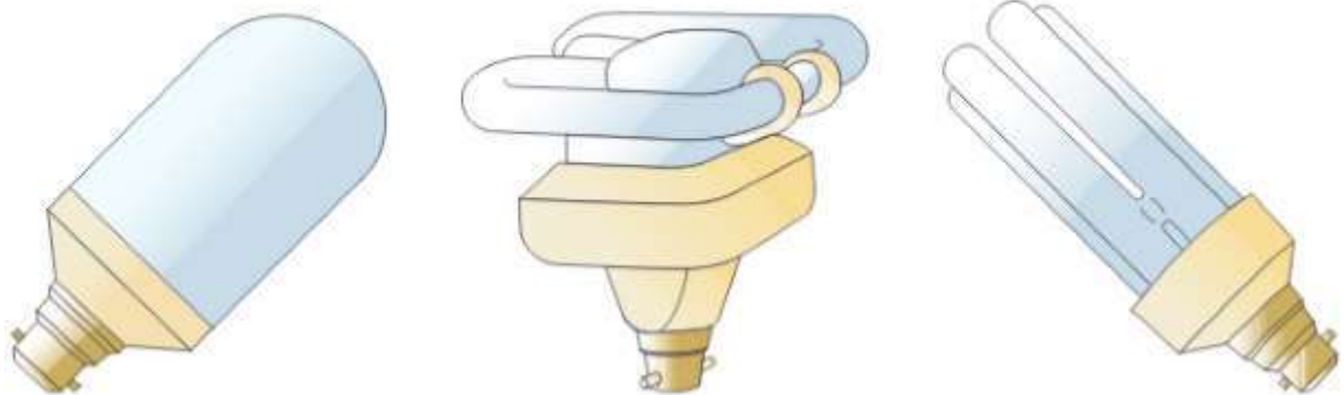
Figure 273 Energy efficient lamps
