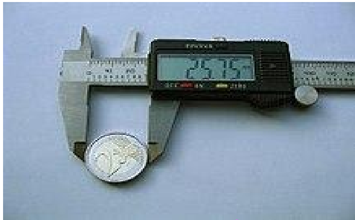
Figure 4: A Caliper for Measuring Length
