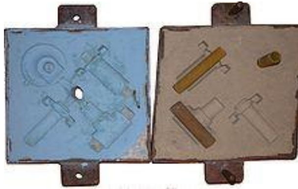
Figure 5: A Sand- Casting Mold
