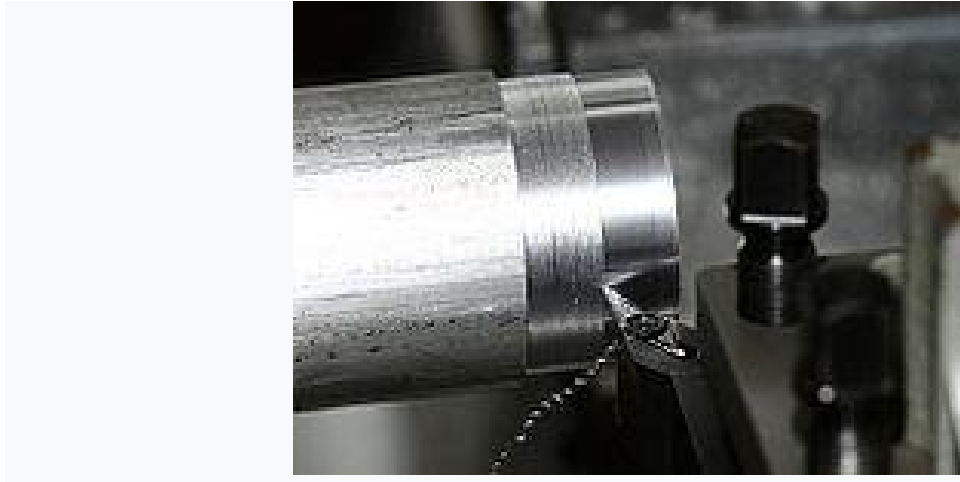
Figure 9: A Lathe Cutting Material from a Workpiece
