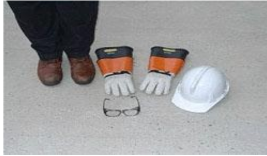
Figure 1: Basic PPE for Electrical Operator
