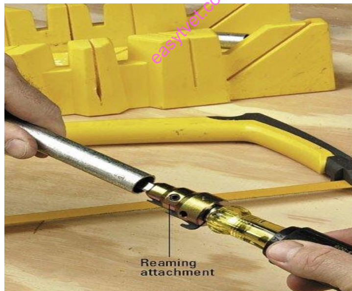
Figure 35: Step 3, Cut Conduit
